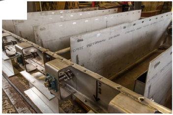
Louver Control Dampers
