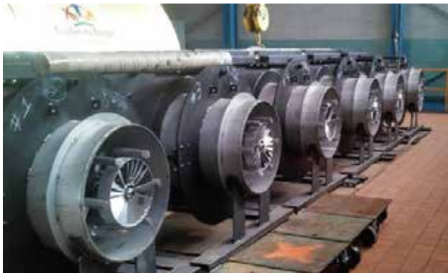
Low-NOx Burners for Multi-Burner Boiler
