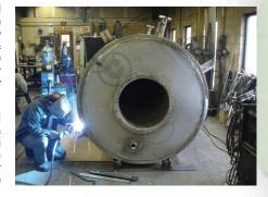
In applications where live energy is being used to heat cold fluids or heat buildings for example, while at the same time hot flue gas is leaving your process or boiler stack, then a cylindrical ConDex can be designed to cost effectively
